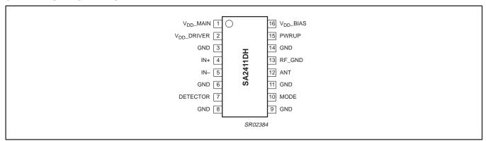
Figure 2. Pin configuration
